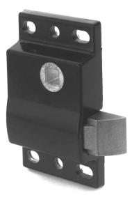
This plunger bolt was designed for lightweight compartment and access doors where low cost slam action latching with L-handle actuation is desired. It features a robust steel plunger bolt for durability and a base mount that allows for ease of installation.
